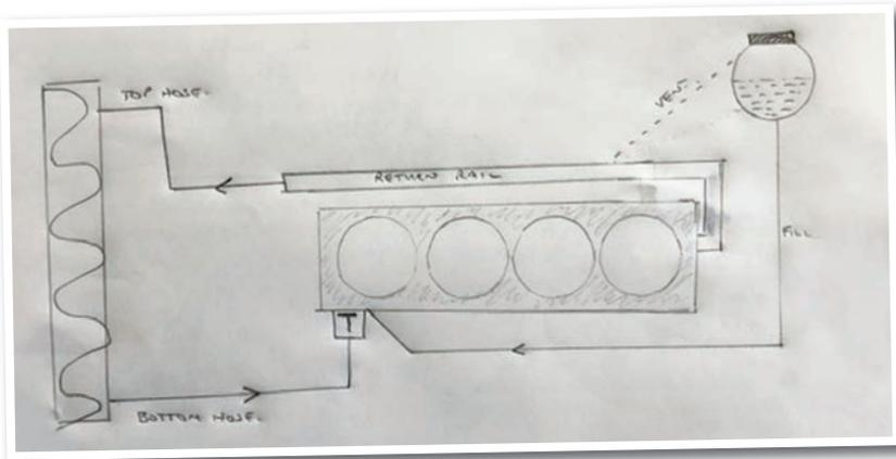
**Diagram 1:** Original 620R cooling circuit (no heater)
