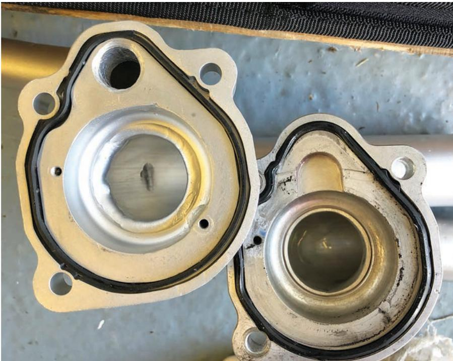
Modified housing (left) with infilled cut-out, new expansion bottle feed and additional mounting point for thermostat alongside original part
